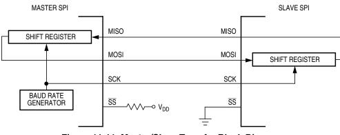
Figure 11-11. Master/Slave Transfer Block Diagram
