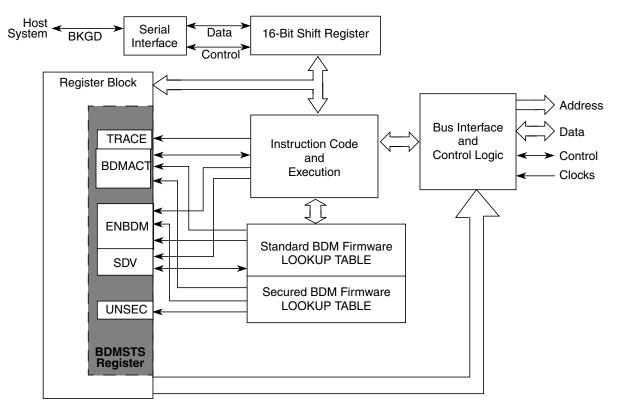
Figure 5-1. BDM Block Diagram
