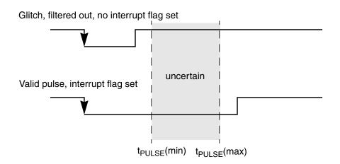
Figure 2-47. Interrupt Glitch Filter (here: active low level selected)
