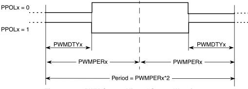
Figure 9-19. PWM Center Aligned Output Waveform
