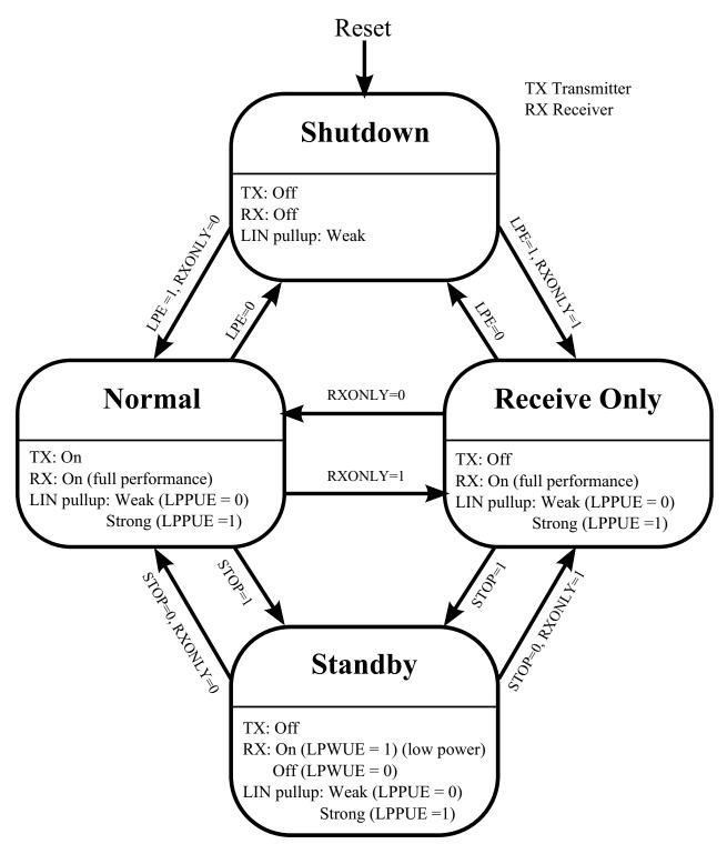
Figure 15-11. LIN Physical Layer Mode Transitions
