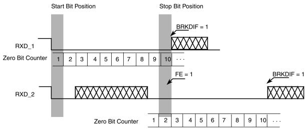
Figure 10-17. Break Detection if BRKDFE = 1 (M = 0)
