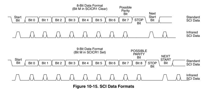
Each data character is contained in a frame that includes a start bit, eight or nine data bits, and a stop bit. Clearing the M bit in SCI control register 1 configures the SCI for 8-bit data characters. A frame with eight data bits has a total of 10 bits. Setting the M bit configures the SCI for nine-bit data characters. A frame with nine data bits has a total of 11 bits.
