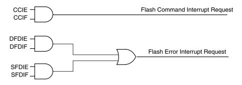
Figure 17-26. Flash Module Interrupts Implementation
