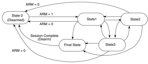
Figure 6-24. State Sequencer Diagram
