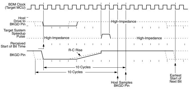
Figure 5-8. BDM Target-to-Host Serial Bit Timing (Logic 1)
