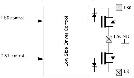
Figure 14-1. LSDRV Block Diagram
