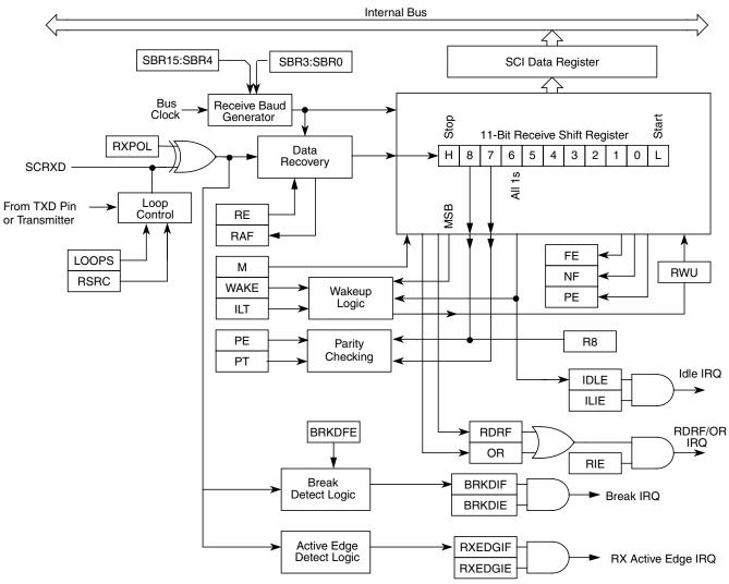
Figure 10-20. SCI Receiver Block Diagram
