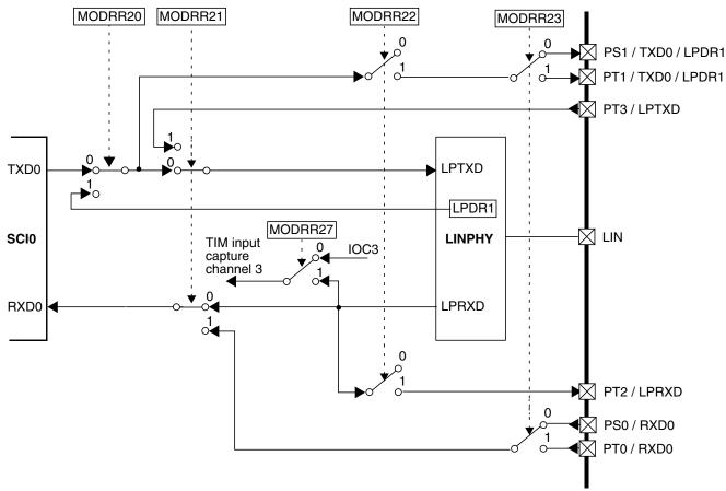
Figure 2-22. SCI0-to-LINPHY Routing Options Illustration
