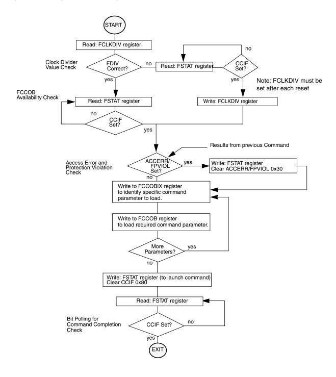
Figure 17-25. Generic Flash Command Write Sequence Flowchart
