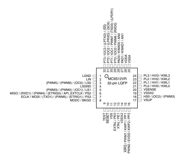
Figure 1-4. MC9S12VR 32-pin LQFP pinout
