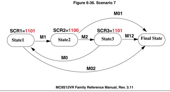
On simultaneous matches the lowest channel number has priority so with this configuration the forking from State1 has the peculiar effect that a simultaneous match0/match1 transitions to final state but a simultaneous match2/match1transitions to state2.
