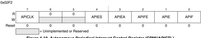
Figure 4-19. Autonomous Periodical Interrupt Control Register (CPMUAPICTL)
