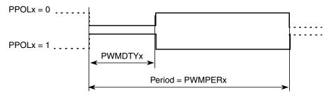
Figure 9-17. PWM Left Aligned Output Waveform
