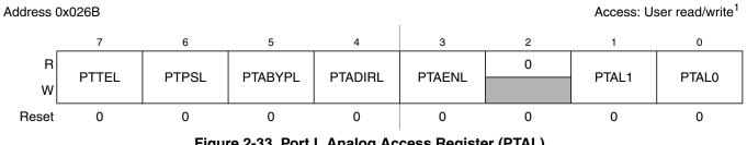
Figure 2-33. Port L Analog Access Register (PTAL)
