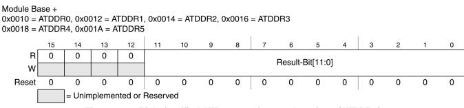
Figure 8-15. Right justified ATD conversion result register (ATDDRn)
