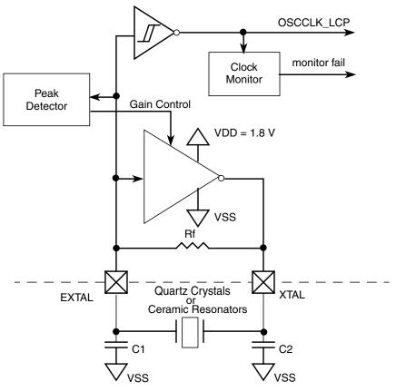
Figure 4-2. XOSCLCP Block Diagram
