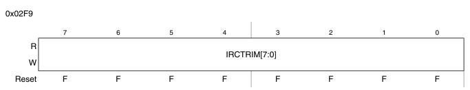
After de-assert of System Reset a factory programmed trim value is automatically loaded from the Flash memory to provide trimmed Internal Reference Frequency  $f_{IRC1M\_TRIM}$ .
