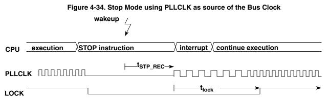
Depending on the COP configuration there might be an additional significant latency time until COP is active again after exit from Stop Mode due to clock domain crossing synchronization. This latency time of 2 ACLK cycles occurs if COP clock source is ACLK and the CSAD bit is set and must be added to the device Stop Mode recovery time  $t_{STP\_REC}$ . After exit from Stop Mode (Pseudo, Full) for this latency time
