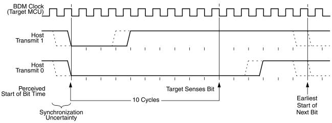
Figure 5-7. BDM Host-to-Target Serial Bit Timing
