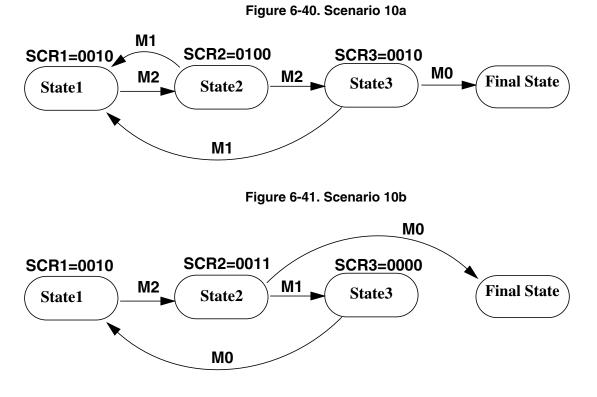
Scenario 10b shows the case that after M2 then M1 must occur before M0. Starting from a particular point in code, event M2 must always be followed by M1 before M0. If after any M2, event M0 occurs before M1 then a trigger is generated.
