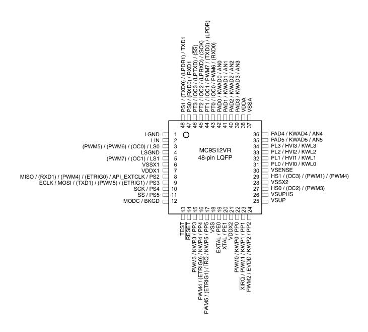
Figure 1-3. MC9S12VR 48-pin LQFP pinout
