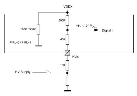
Figure 2-48. Digital Input Read with Pullup Enabled
