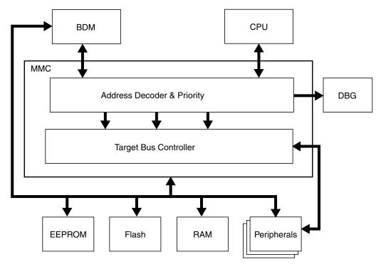
Figure 3-1. S12GMMC Block Diagram
