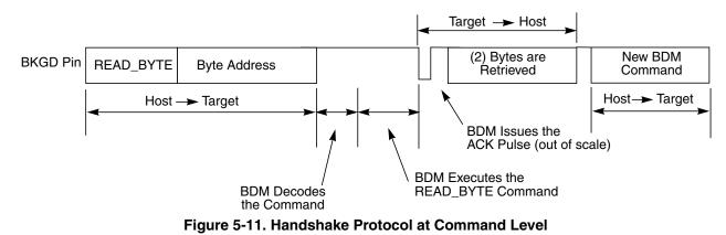
Differently from the normal bit transfer (where the host initiates the transmission), the serial interface ACK handshake pulse is initiated by the target MCU by issuing a negative edge in the BKGD pin. The hardware handshake protocol in Figure 5-10 specifies the timing when the BKGD pin is being driven, so the host
