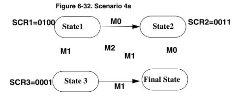
This scenario is currently not possible using 2 comparators only. S12SDBGV2 makes it possible with 2 comparators, State 3 allowing a M0 to return to state 2, whilst a M2 leads to final state as shown.
