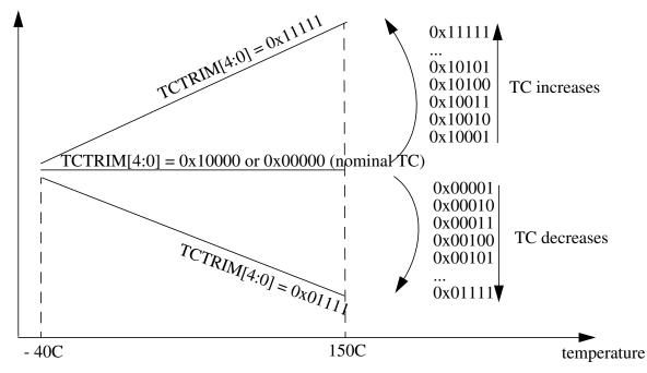
Figure 4-29. Influence of TCTRIM[4:0] on the Temperature Coefficient
