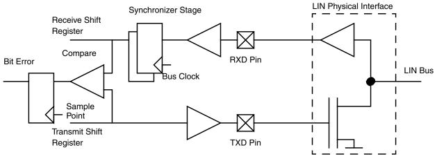
Figure 10-18. Collision Detect Principle
