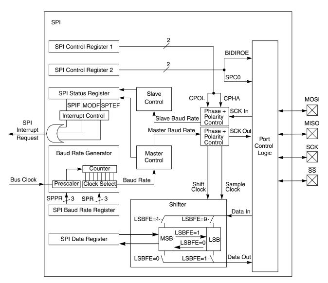
Figure 11-1. SPI Block Diagram
