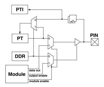
Figure 2-45. Illustration of I/O pin functionality
