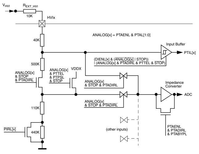
Figure 2-46. HVI Block Diagram
