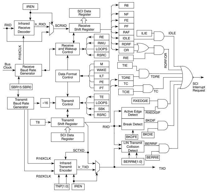
Figure 10-14. Detailed SCI Block Diagram
