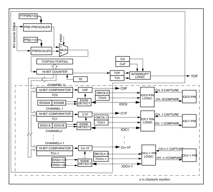
Figure 12-22. Detailed Timer Block Diagram
