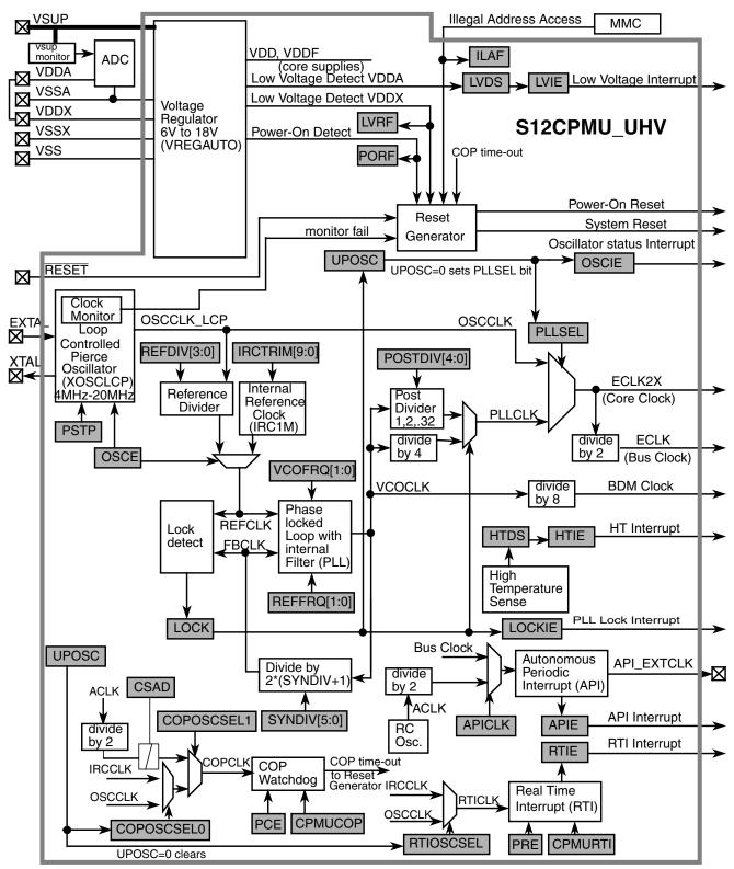
Figure 4-1. Block diagram of S12CPMU\_UHV
