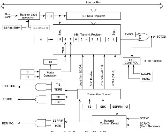
Figure 10-16. Transmitter Block Diagram
