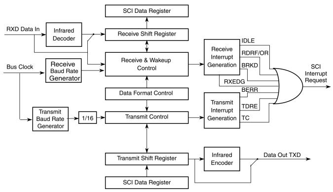
Figure 10-1. SCI Block Diagram
