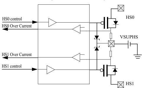
Figure 13-1. HSDRV Block Diagram
