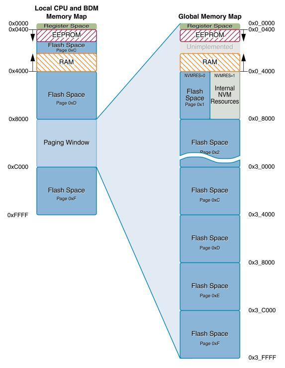
Figure 3-11. Local to Global Address Mapping
