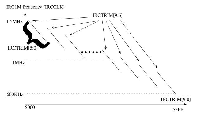
Figure 4-28. IRC1M Frequency Trimming Diagram
