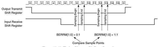
Figure 10-19. Timing Diagram Bit Error Detection
