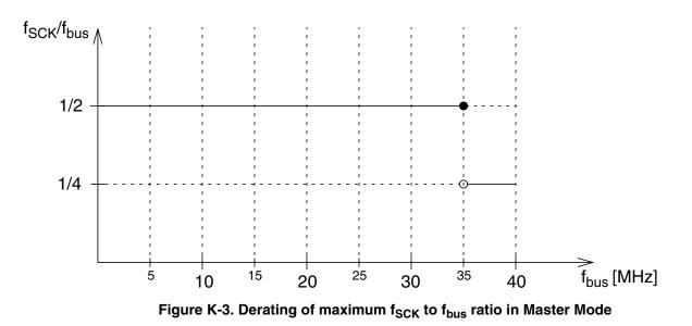
In Master Mode the allowed maximum  $f_{SCK}$  to  $f_{bus}$  ratio (= minimum Baud Rate Divisor, pls. see SPI Block Guide) derates with increasing  $f_{bus}$ , please see **Figure K-3.**
