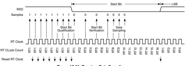
Figure 10-21. Receiver Data Sampling
