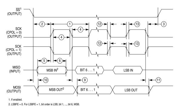
Figure K-1. SPI Master Timing (CPHA=0)
