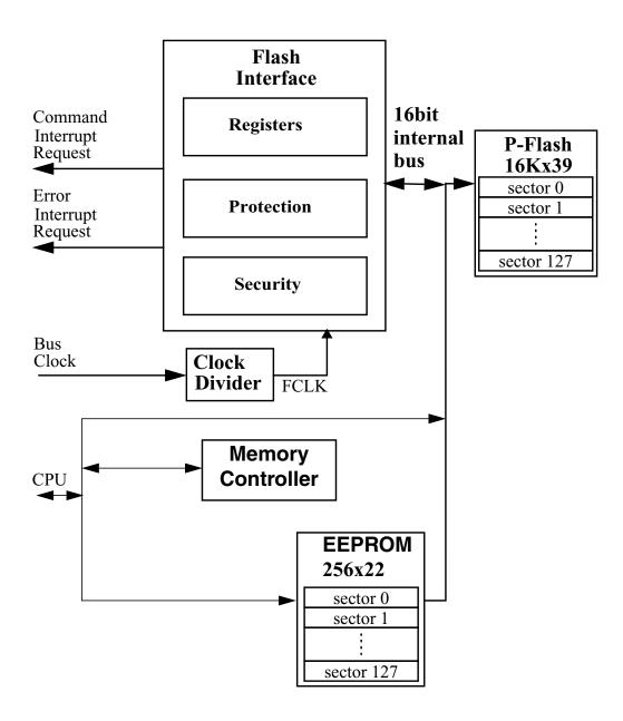
Figure 17-1. FTMRG64K512 Block Diagram
